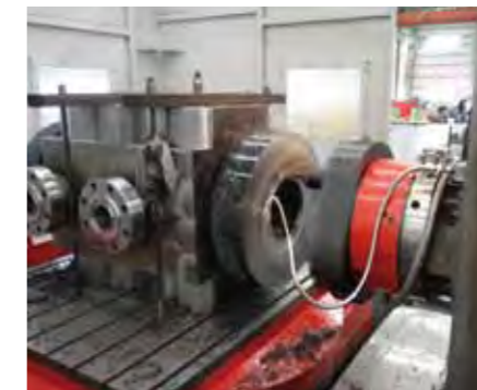
Turning big diameter hole by NC facing head(opt.)
