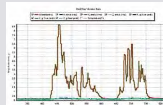
Fig.1 Vibration report without compensation
