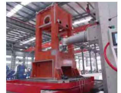
A press brake machine frame (by angle head, opt.)
