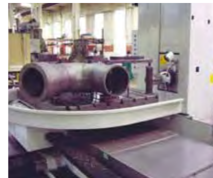
Deep boring of inner pipe hub
