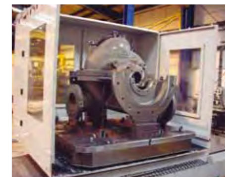
Milling and boring a fire-fight equipment
