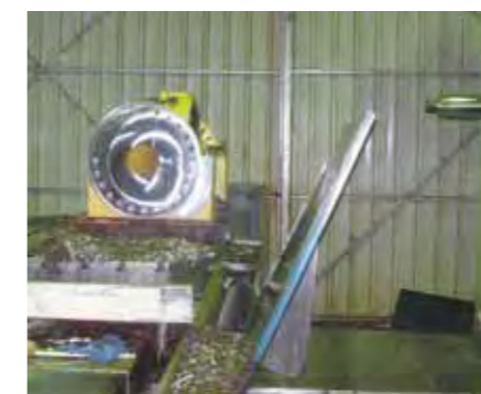
Boring and drilling truck wheel axle
